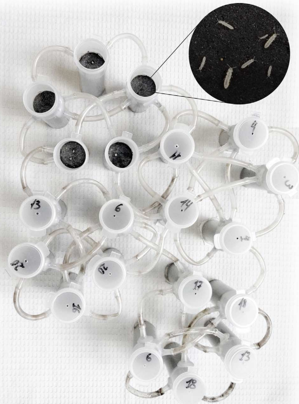
Fig. 1. Top-down view of one of the replicate experimental networks. The network comprises 20 vials representing nodes or habitat patches inhabited by a local population of the arthropod species F. candida [pictured with a stereomicroscope, size 1 to 2 mm (inset)]. These nodes are connected by tubular corridors through which the arthropods can move, creating a metapopulation occupying a network of habitat patches.
